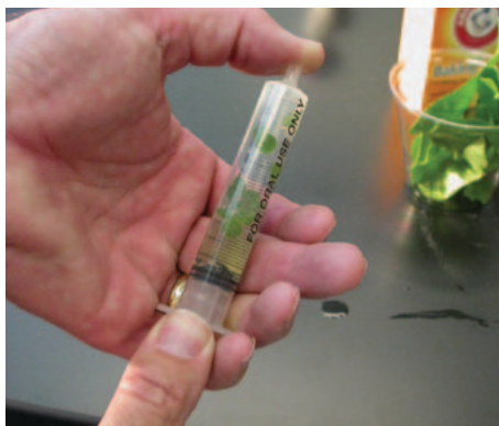
Figure 6a. Creating a Vacuum in the Plunger
