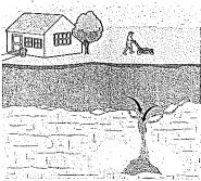
Erosion carves out cavities in the bedrock beneath the soil. Sediment flows down into a cavity through cracks in the bedrock.
