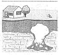
The cavity grows larger over time, but remains undetectable from the surface.
