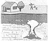
Sediment keeps flowing into the cavity, but some of the soil particles catch against each other and form an arch over the hole.
