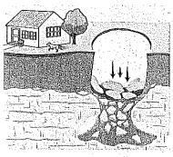
Eventually, the roof over the cavity collapses, creating a sudden and dramatic sinkhole.
